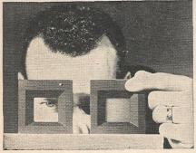
Clear and frosted. The only difference between the two windows is that an electric field has been applied to the one on the right, causing the liquid crystals to become opaque.
