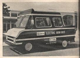
lead-acid cells. The vehicle, made by Battronic Truck Corp., Boyertown, Pa., uses SCR controls to provide fast starts, smooth operation and maximum range. Truck versions of this vehicle are also available.
