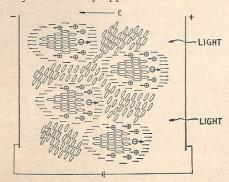
lons in transit cause disruptions in liquid crystal that result in turbulence that turns liquid white. The ions are created when an electric field is applied to the liquid crystals.
